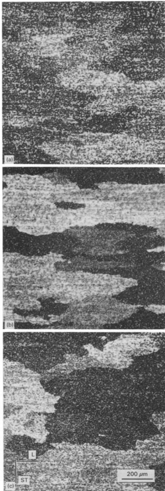
Figure 12 Effect of solution heat treatment on the microstructure of reinforced hot rolled sheet; (a) Al-4.35%Cu; (b) Al-4.7%Cu-0.12%Zr; and (c) Al-6%Cu.
